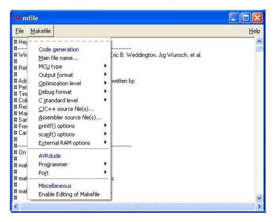
The Makefile is saved under the name Makefile (without extension i.e. .EXE for example) in the same folder into also the file main.c ("the program code") is put down. More detailed explanations for the function of Makefiles are in the following to section <a href="Exploring Makefiles"><u>Exploring Makefiles</u></a>.
