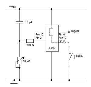
The port pin of the microcontroller on output one configures (in the example DDRD /= (1 << PD3)) and this output on logic 1 ("High", PORTD /= (1 << PD3)) switched, the same potential **VCC** rests and the condenser thus unloaded against both "plates" of the condenser. (Sounds amusingly, with **Vcc** unloaded, is at both sides of the condenser the same potential fits however in such a way, there and thus a difference of potential of 0V exists => condenser is unloaded).
