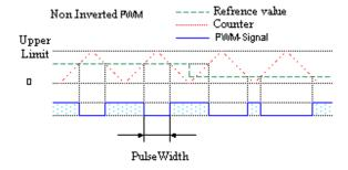
Oh, nearly I would have forgotten. The generated **PWM-signal** spent at the output Compare pin **OC1 of the** timer and unfortunately to know we therefore also with AT90S2313 only an individual **PWM-signal** with this method to generate. Other AVR types order over up to four PWM outputs.
