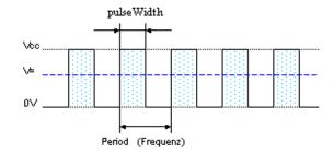
This square wave voltage has now a geometrical average value, which is depending upon Pulse width smaller or larger.
