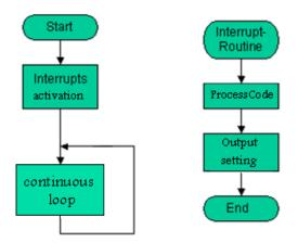
One sees that the interrupt routine runs off quasi parallel to the main program. There we only one CCU have are natural it no genuine parallelism, but the main program is interrupted with the arrival of an interrupt, the interrupt routine is implemented and to it only again to the main program returns.
