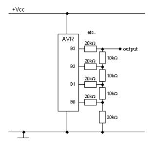
Naturally if possible details of resistors should be used, thus not necessarily such with a tolerance of 10% or more. Further it is advisable to strengthen depending upon application output current over an operation amplifier.
