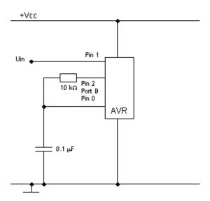
The principle of the measurement is now quite analog to the preceding. By creation of a LOW level at pin 2 the condenser is first once unloaded. Also here it must be paid attention to the fact that the discharge process lasts sufficient long.
