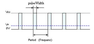
If we filter now this pulsating output voltage still over an RC element "smooth", then have we already appropriate DC voltage produced.
